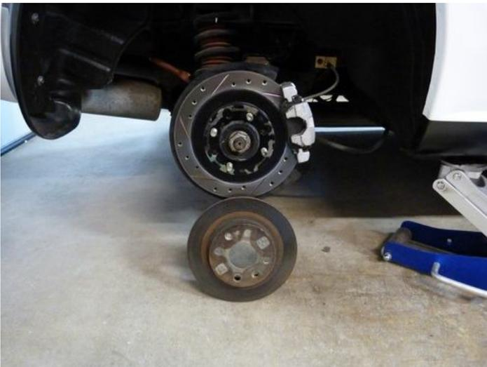
Attached is a picture of the upgraded brakes compared to the old, smaller rotor that was replaced. The improvement in braking capability, pedal feel, and driver confidence was well worth the minimal cost of the project. If you have any questions, please don't hesitate to contact me.
